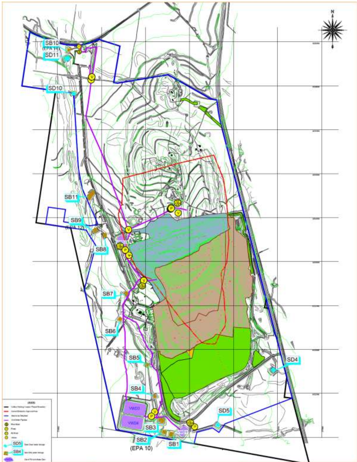
Figure 2.5 Void Water Management System Plan
